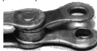
Chain with pin completely removed (avoid this)
